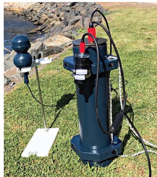
The real-time hydrophone unit costs about $5,000, making it affordable for management agencies and NGOs. Photo: Middy Khong
